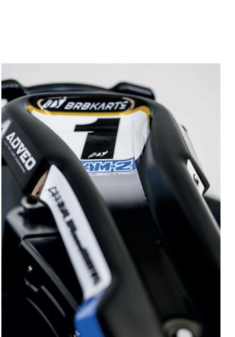
Thanks to the optimization of the design and when working with light materials, a weight that can vary between 175 and 185 kg has been achieved, depending on the extras, a factor that translates into less consumption of batteries, tires, lightness in the direction and lower impact force in case of collisions
